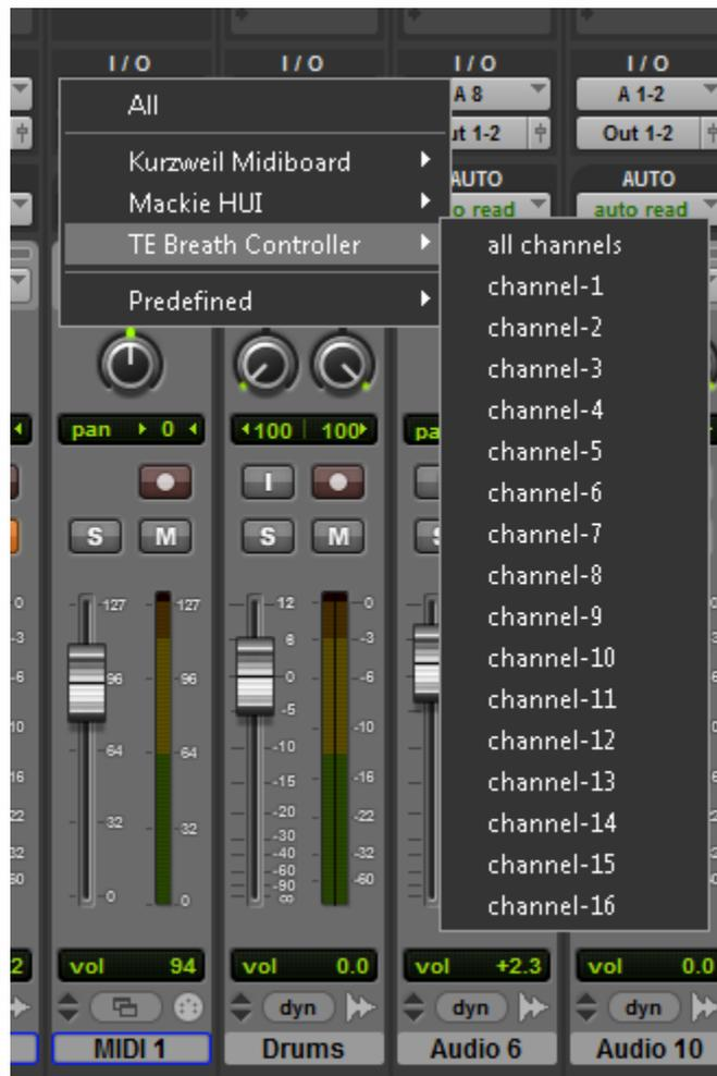
Choose **channel-1**, which is the default channel for the BC “out of the box” or choose **all channels**. You can also use the **TEC Configuration Utility** to change the input channel of the BC.
